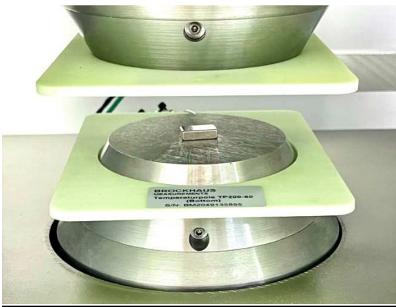
5: MIM magnet in hysteresis graph for magnetic characterization.
